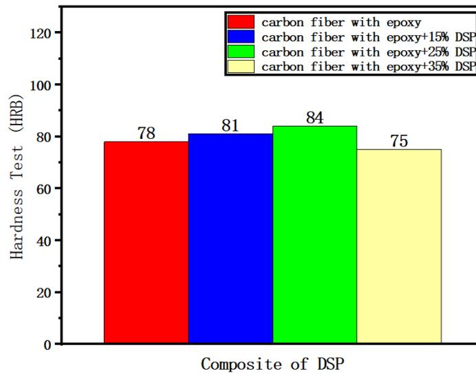
**Fig. 11** Shore hardness number HRB in different composition
