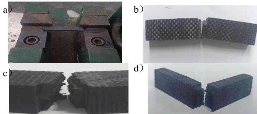
**Fig. 10** Sample Impact: a) 0% DS before the test, b) 15% DS after the test, (c) 25% DS after the test, and d) 35% DS before the test
