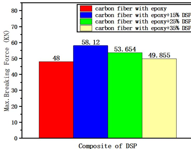
**Fig. 5** Maximal breaking force for different composites
