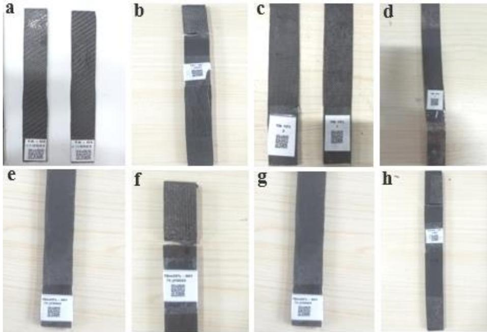
**Fig. 6** Sample tensile test: a) and b) 0% DS before and after the test; c) and d) 15% DS before and after test; e) and f) 25% DS before and after the test; g) and h) 35% DS before and after the test
