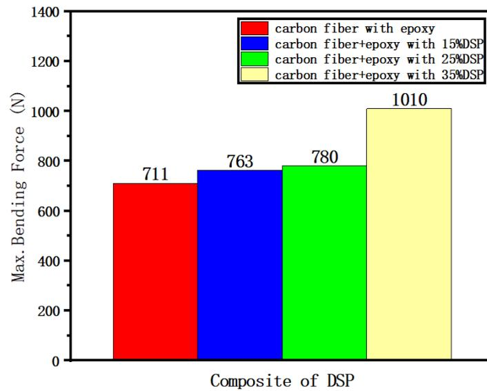
**Fig. 7** Maximum bending force in different composites
