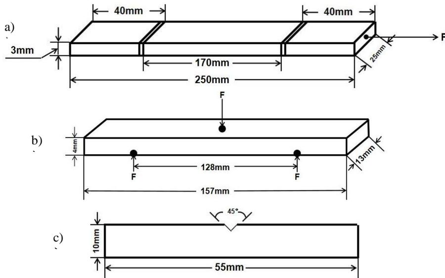
**Fig. 3** Sample dimensions in: a) tensile; b) bending; and c) impact test
