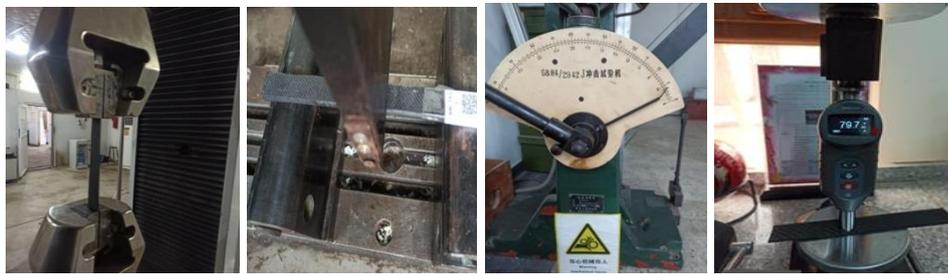
**Fig. 4** From left to right: tensile device, binding device, impact device, and hardness device
