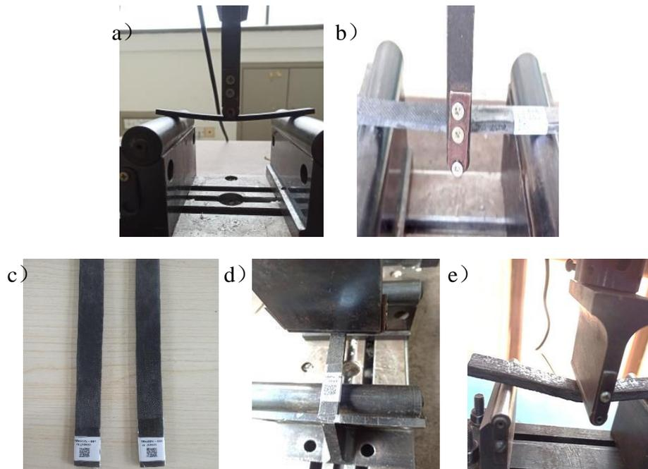
**Fig. 8** Sample bending test: a) 0% DS after the test, b) 15% DS during the test, c) 25% DS before the test, d) 35% DS under the test, and e) 35% DS after the test
