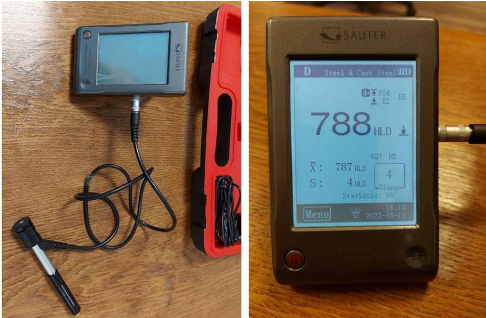
**Fig. 9** Hardness measurement device
