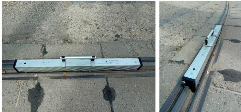
**Fig. 4** Rail straight measurement device
