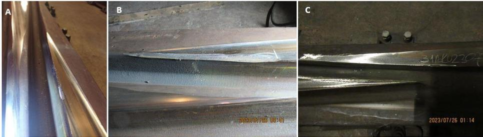
**Fig. 1** Repair of a turnout frog from Hadfield steel. A – defect, B – preparation, C – welded structure
