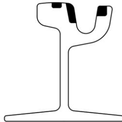
**Fig. 2** Build-up welding on grooved rails to reduce wear
