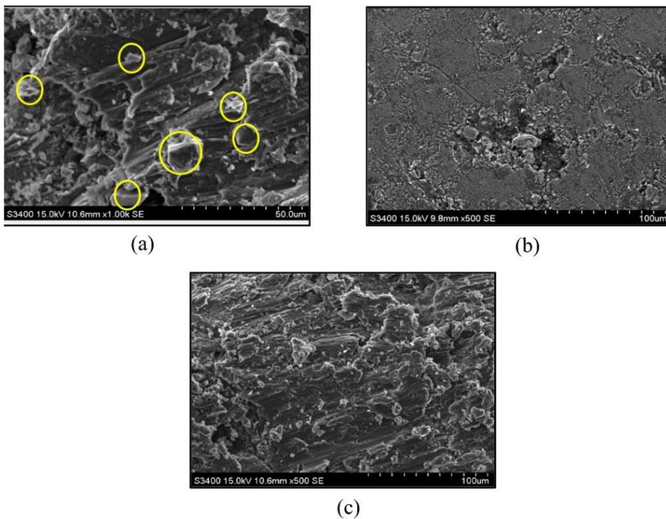
**Fig. 12** SEM images of (a) Al-MMC after wear test with SiC particles in the matrix (b) microstructure of subsurface of laser-treated Al-MMC (c) microstructure of laser-treated Al-MMC with clad layers
