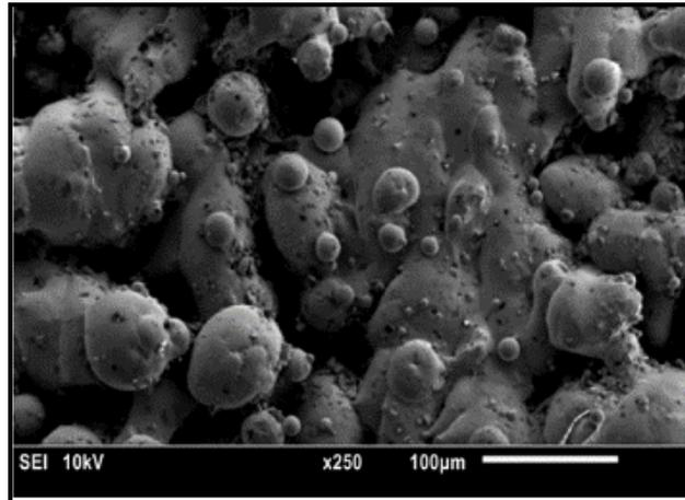
**Fig. 5** Traces of recast nodules of matrix material
