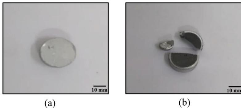
**Fig. 10** Al-MMC sample before, and after wear testing, the dark color shows the rubbing of SiC particles still embedded in the matrix.
