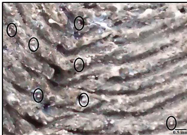
**Fig. 6** SEM image of laser-treated Al-MMC, showing fine spheroids
