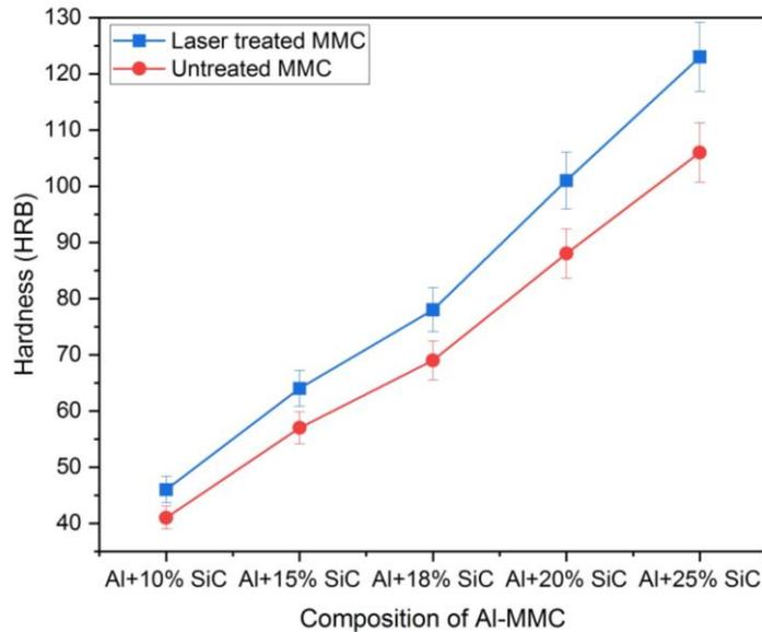
**Fig. 8** Comparisons of the hardness of laser treated and untreated MMC
