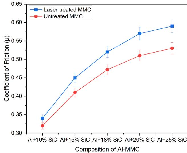
**Fig. 13** Variation of coefficient of friction for laser-treated and untreated Al-MMC
