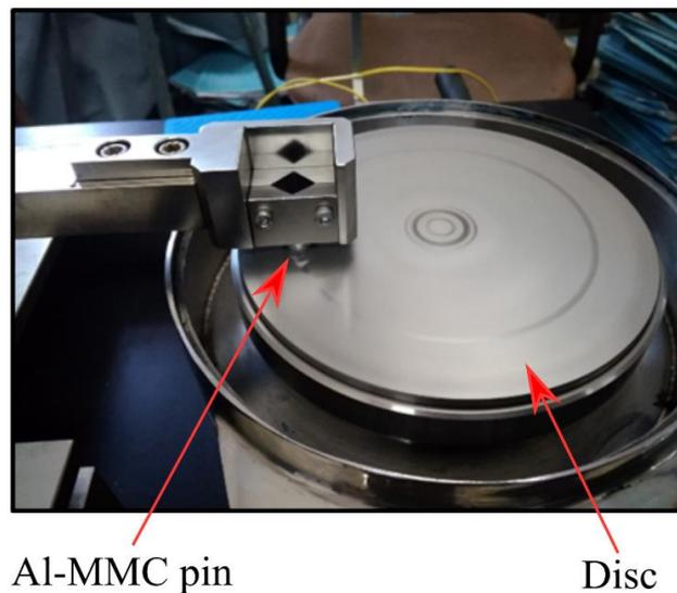
**Fig. 4** Wear testing of Al-MMC on Pin-on-Disc setup
