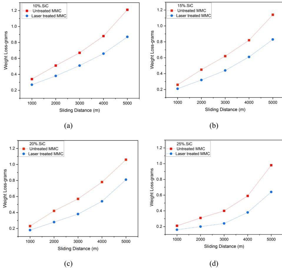
**Fig. 11** Wear of laser-treated and untreated Al-MMC with (a) 10% SiC (b) 15% SiC (c) 20% SiC (d) 25% SiC at 40 N load
