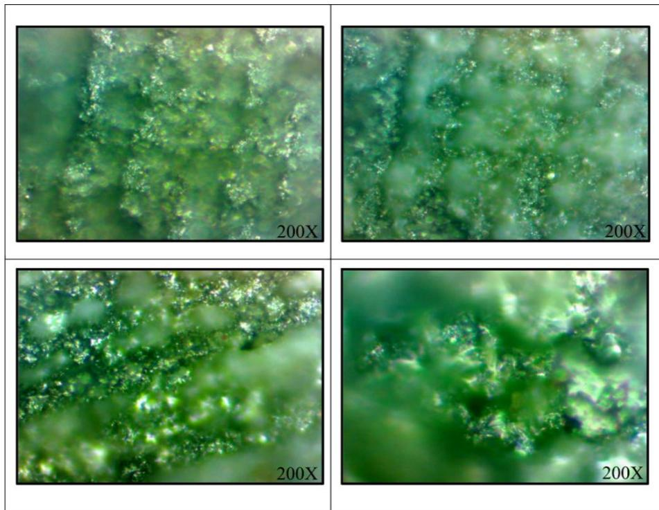
**Fig. 9** Micrographs of the laser-treated surface of Al-MMC, showing the distinct alternate region
