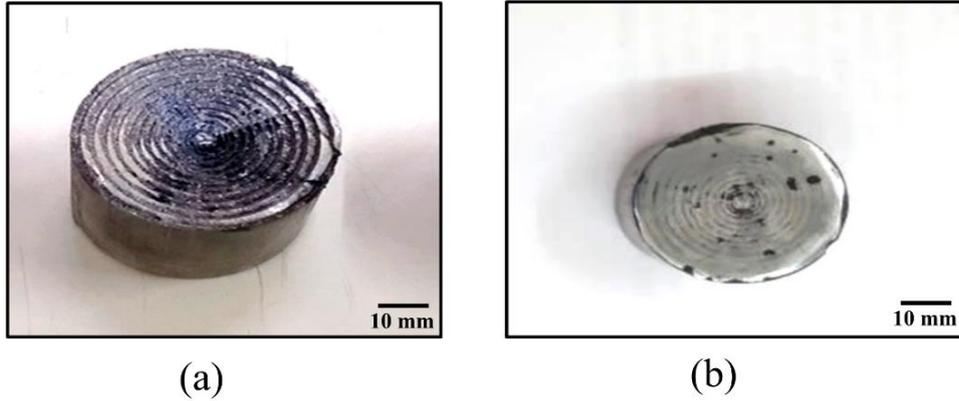
**Fig. 7** Traces of Laser tracks, showing the effect of the laser beam (a) on the surface (b) laser tracks at 3 mm depth
