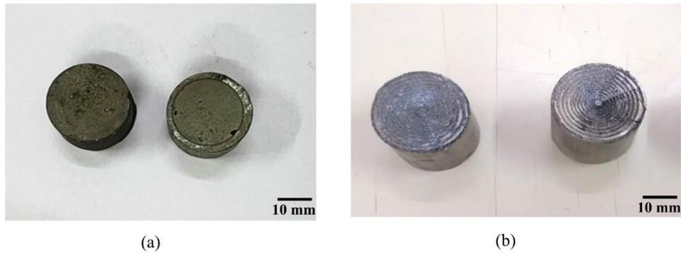
**Fig. 3** Al-MMC samples (a) before (b) after the laser treatment
