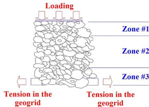
**Fig. 1** The zones of the interlocking effect in a granular material due to a planar geogrid layer (on the basis of [33,34])
