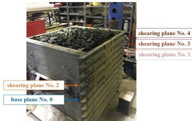
**Fig. 3** Marking of shearing planes [8]
