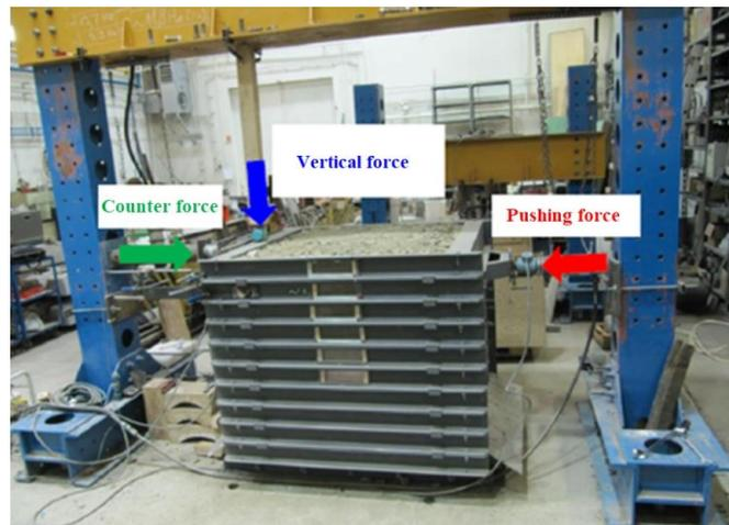
**Fig. 2** The measuring principle of the multi-level shear box [8]
