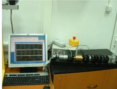
**Fig. 8** Photo of nonlinear servo system experimental setup in authors' laboratories [22]
