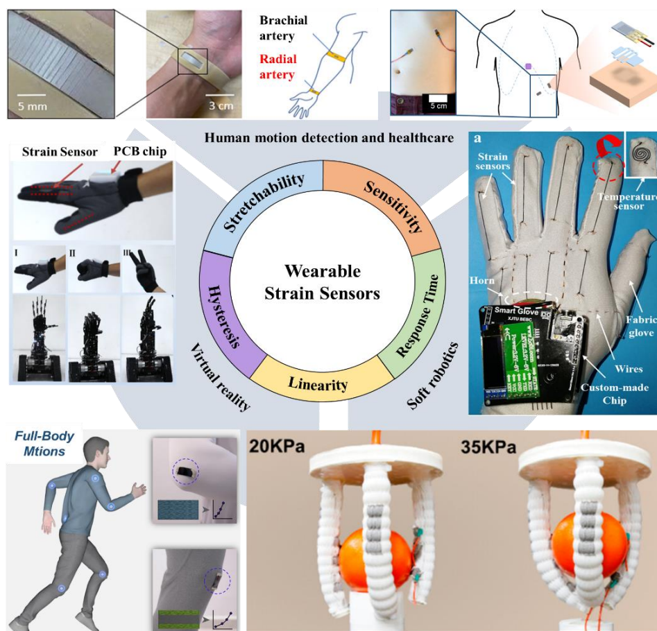
Fig. 1 State-of-the-art flexible, wearable strain sensors made of nanomaterials and polymer composites. Reprinted with permission from [11], copyright 2023 American Chemical Society. Reprinted with permission from [18], copyright 2022 Springer Nature. Reprinted with permission from [19], copyright 2021 Wiley. Reprinted with permission from [20] under the Creative Commons Attribution 4.0 International (CC BY 4.0) License. Reprinted with permission from [21], copyright 2020 American Chemical Society.
