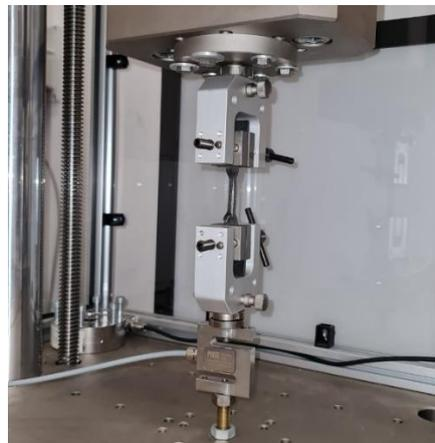
**Fig. 4** Tensile testing setup
