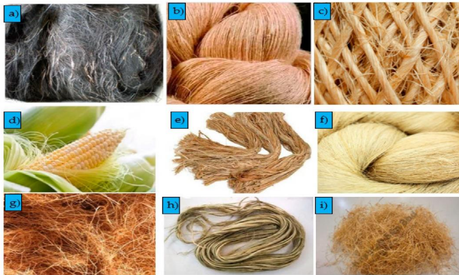
Fig. 10 Commonly used natural fiber in ballistic applications (a) Sugar palm fiber, (b) Pineapple fiber, (c) Hemp fiber, (d) Corn fiber, (e) Jute fiber, (f) Flax fiber, (g) Coir fiber, (h) Kenaf fiber, (i) Empty fruit bunch fiber [91]
