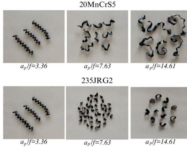
**Fig. 6** Chip morphology as a function of chip slenderness ratio
