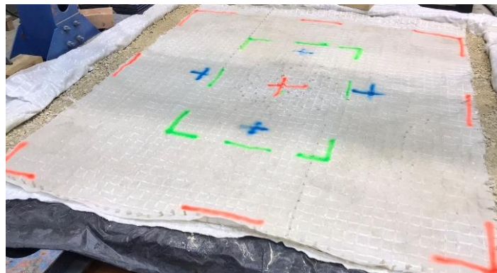
Fig. 2 Set-up of the protection layer, border signs of the materials
