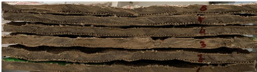
Fig. 14 Specimens Nr. 1-6 after the four-point bending test
