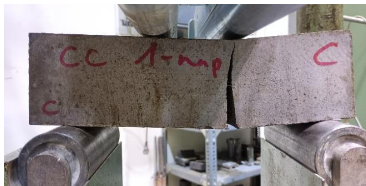
Fig. 6 The set-up of the four-point bending test and the broken CC specimen
