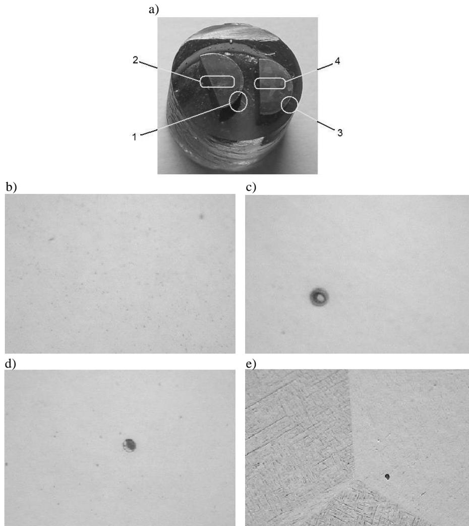
**Fig. 6** (a) Samples B2 and C2 from the billet 2 showing the fields analyzed: on the left the area taken from the center of the billet and on the right took from its bottom; (b) field 1, apparently with no globular formations, 400x; (c) and (d) field 2 and 3, respectively, with one globular formation with a phase inside, 400x; (e) field 4, detail of grain boundaries, 400x
