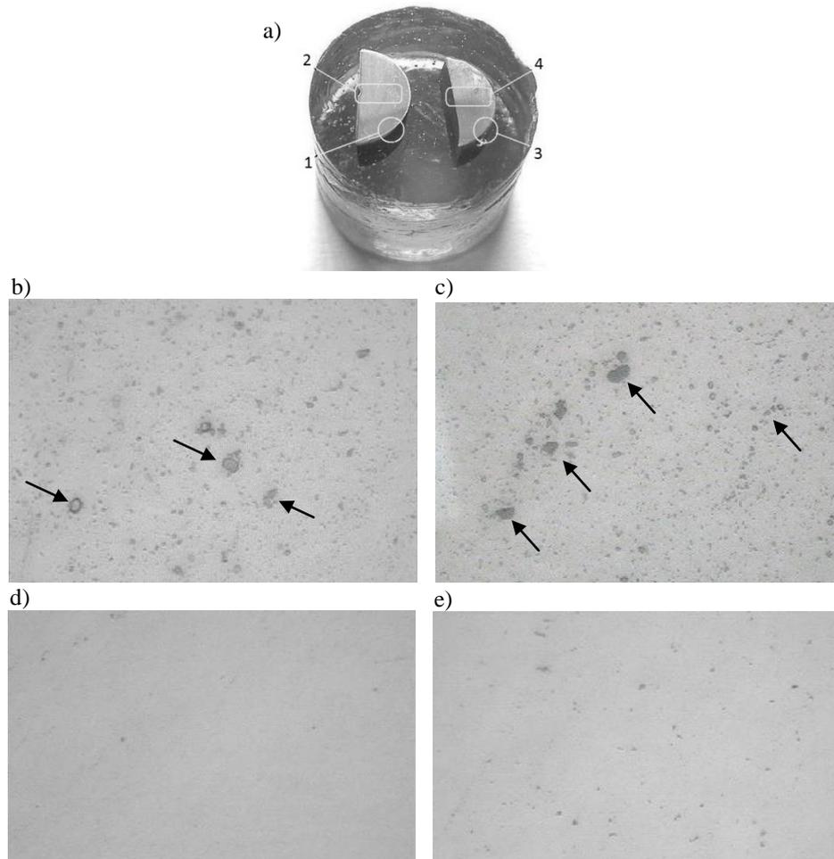
**Fig. 4** (a) Samples B1 and C1 from the billet 1 showing the fields analyzed, 400x; (b) field 1, detail of globular formations; (c) field 2, detail of globular formations; (d) field 3 and (e) field 4
