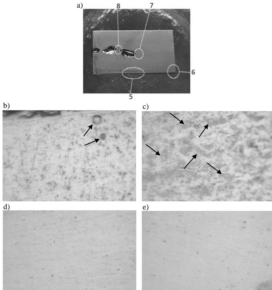
**Fig. 5** (a) Sample A1 from billet 1 showing the fields analyzed; (b) field 5, detail of globular formations, 400x; (c) field 6, detail of globular formations, 400x; (d) and (e) field 7 and 8, respectively with no apparent globular formation, 400x
