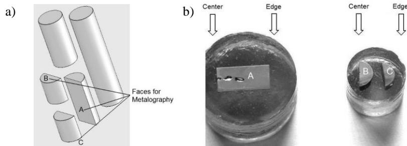
**Fig. 2** (a) parts for OM evaluation showing the faces analyzed nominated as A1, B1 and C1 for the billet 1 and A2, B2 and C2 for the billet 2; (b) Left: sample longitudinal to the billet axis; right: sample transversal to the billet axis.
