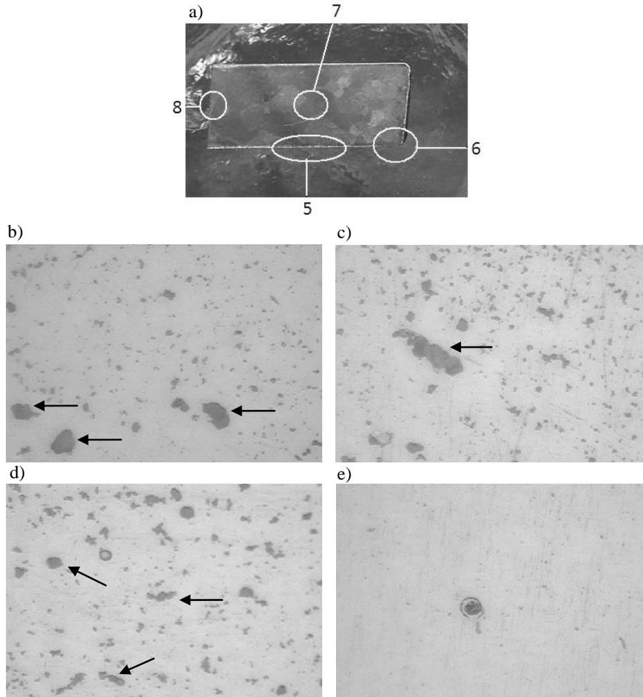
**Fig. 7** (a) Sample A2 from billet 2 showing the fields analyzed: on the left side the center of the billet and the right side its bottom; (b), (c) and (d) field 5, 6 and 7, respectively, showing globular formations, some in a visible coalescence phase (arrows), 400x; (e) field 8 showing one globular formation with a phase inside, 400x
