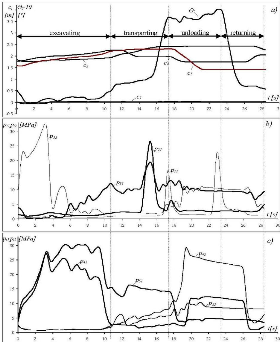
**Fig. 2** Measured quantities of the state of the excavator: a) movement of the rotating mechanism, angle of the platform rotation and motions of manipulator hydraulic cylinders, b, c) pressures in the excavator drive mechanism actuators
