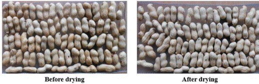
**Fig. 5** Photograph of groundnut sample before and after drying
