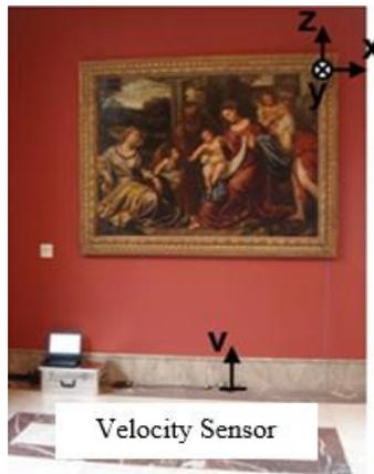
**Fig. 6** Measurement setup for the investigations of the vibration excitation of the suspension system: steel hooks (oil painting “The Holy Family” by Luciano Podormo, Bode-Museum, Berlin) [23]
