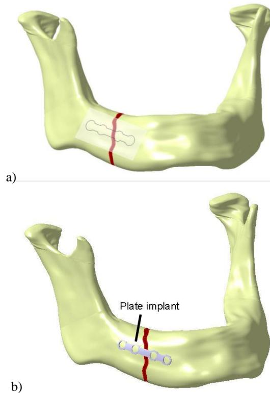
**Fig. 4** Construction process of the personalized plate implant: a) Construction plane and outer contour of the tension band plate; b) Solid model of the tension band plate implant with 4 holes
