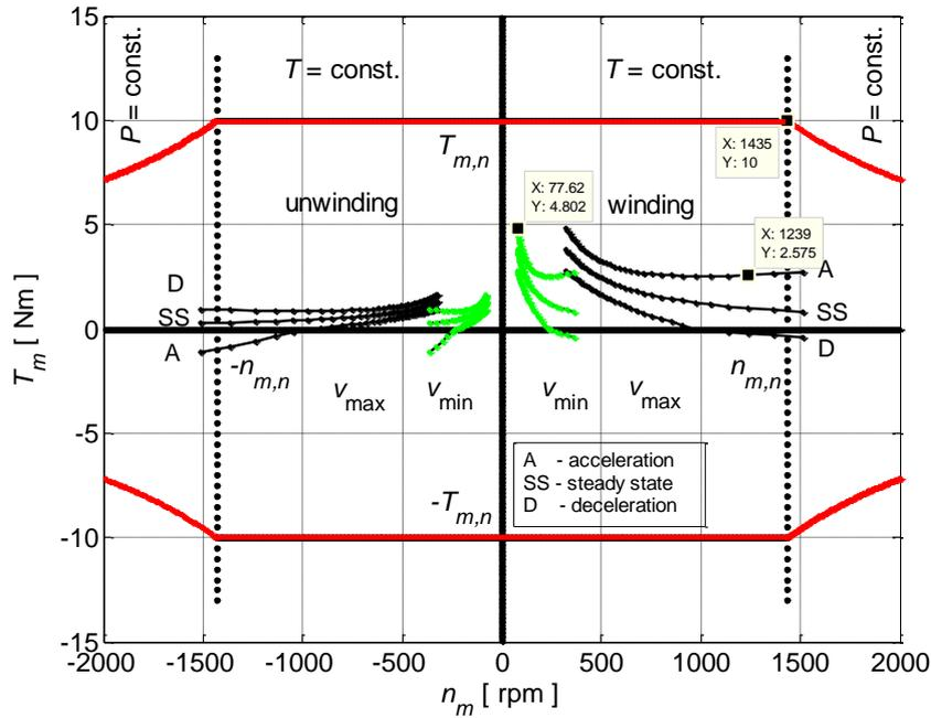
**Fig. 6** Torque-speed characteristics for  $v_{max}$  (black) and  $v_{min}$  (green) with possible working area for motor (red)
