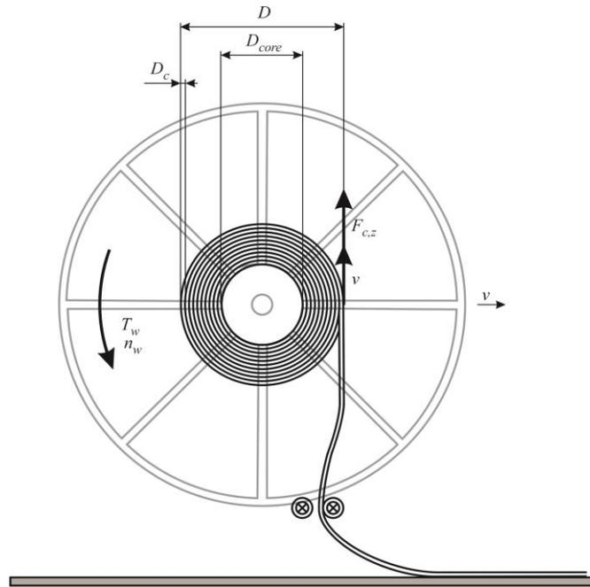
**Fig. 1** Schematic view of the cable reel
