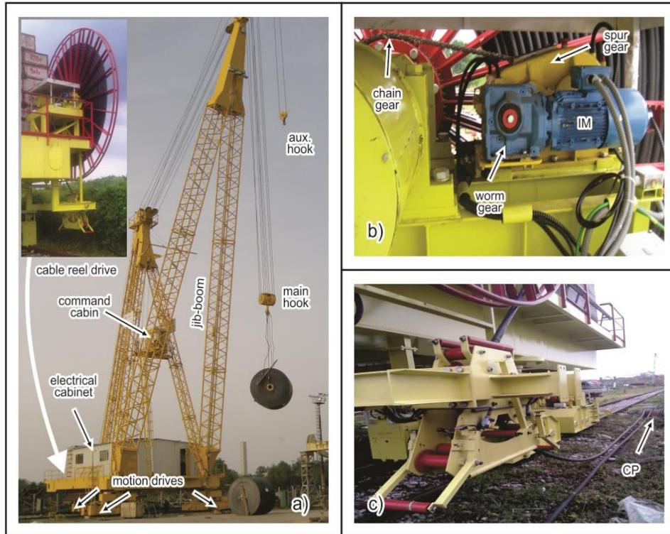
**Fig. 4** Derrick crane DK 004 with: a) indicated drives, b) cable reel drive components, c) terminal box of cable reel
