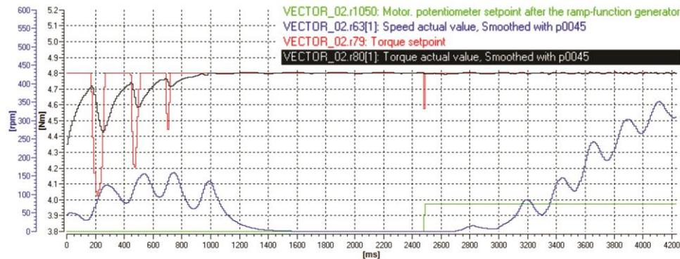
**Fig. 7** Experimental results – cable winding, acceleration regime
