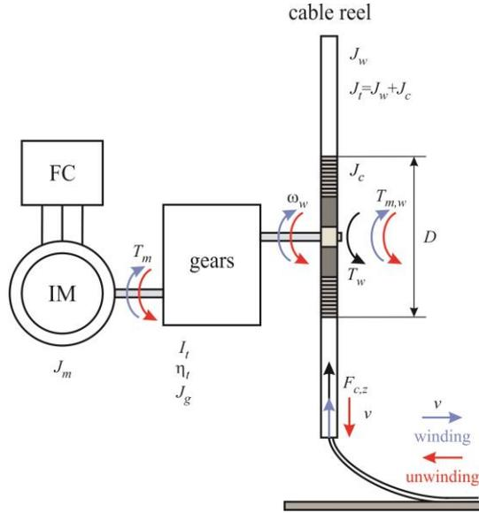
**Fig. 2** Schematic view of the cable reel drive - winding/unwinding operation
