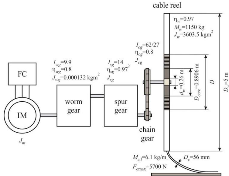
**Fig. 5** Principal block diagram of the cable reel drive on derrick crane DK 004
