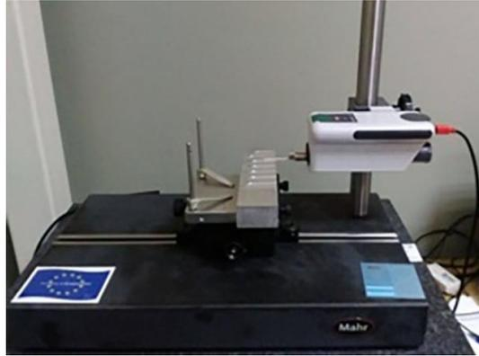
**Fig. 3** Mahr profilometer for measuring surface roughness
