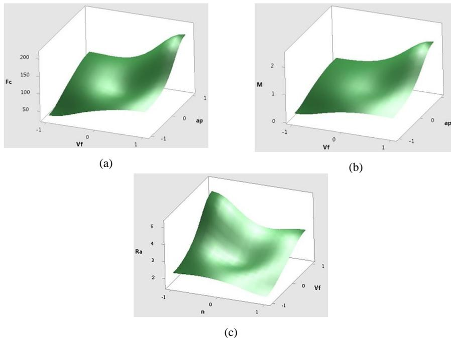
**Fig. 5** 3D surface plots of a) cutting force, b) moment and c) surface roughness
