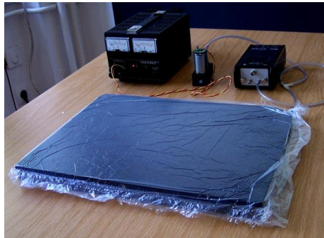
Fig. 4 Sound-insulating experimental panel enclosed in an airtight package, vacuum pump and indicator in the rear
