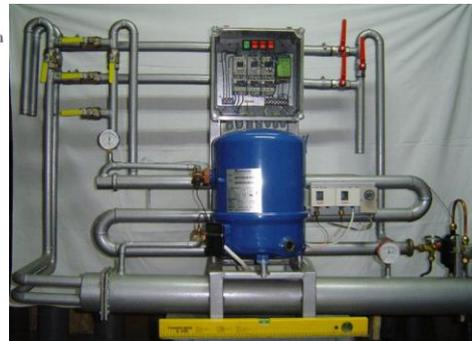
**Fig. 2** Photo of the heat pump with coaxial evaporator and shell-tube condenser
