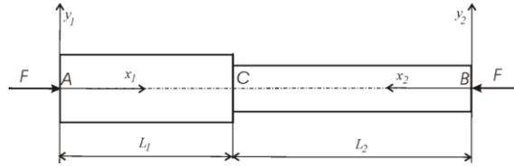
**Fig. 2** The coordinate system and notation for the stepped beam
