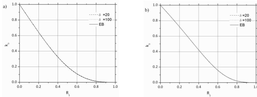
**Fig. 12** Variation of CLP with  $R_1$  for cl-fr beam and  $\theta_2 = 0.8$ : a) type 1, b) type 3
