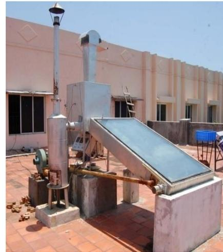
**Fig. 2** Perspective view of the hybrid solar dryer
