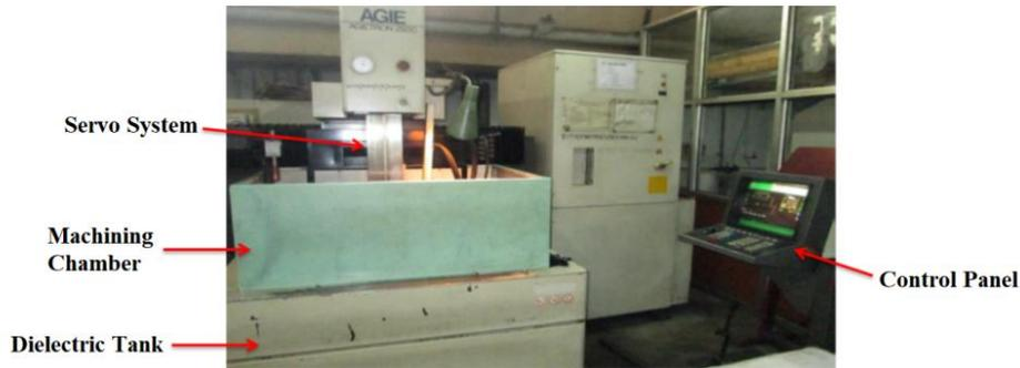
**Fig. 2** EDM set-up
