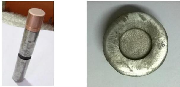
**Fig. 3** Round copper tool and machined component (5 mm depth and 20 mm dia.)
