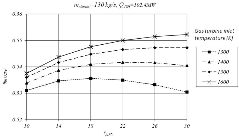
**Fig. 4** Thermal efficiency as a function of the compression ratio ( $r$ ) and the temperature of exhaust gases entering the gas turbine for 130 kg/s steam production and 102.4 MW heat output
