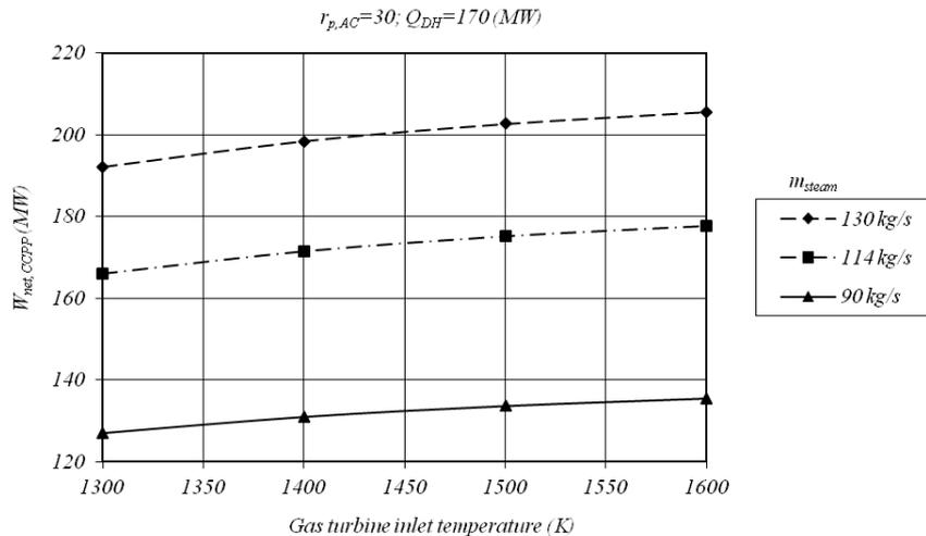
**Fig. 14** Electric power as a function of the temperature of exhaust gases entering the gas turbine, for the nominal heat output 170MW and compression ratio of  $r_{p,AC} = 30$
