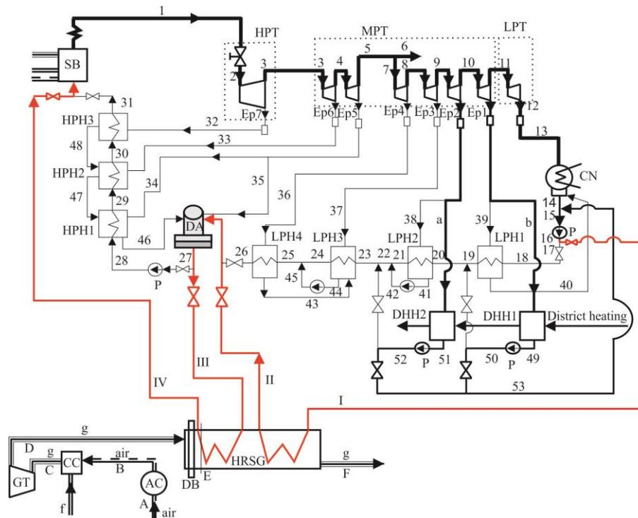
**Fig. 1** Schematic flow diagram of a combined cycle power plant
