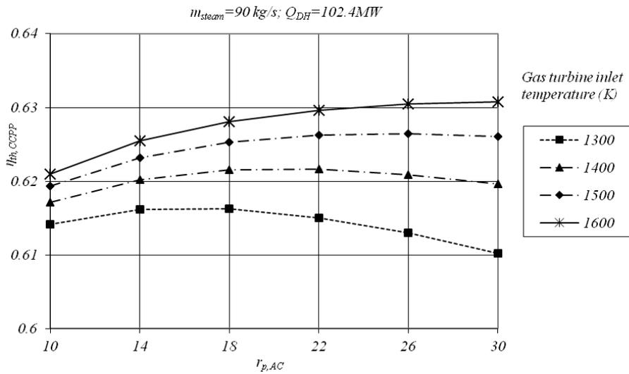
**Fig. 10** Thermal efficiency as a function of the compression ratio ( $r$ ) and the temperature of exhaust gases entering the gas turbine for 90 kg/s steam production and 102.4 MW heat output
