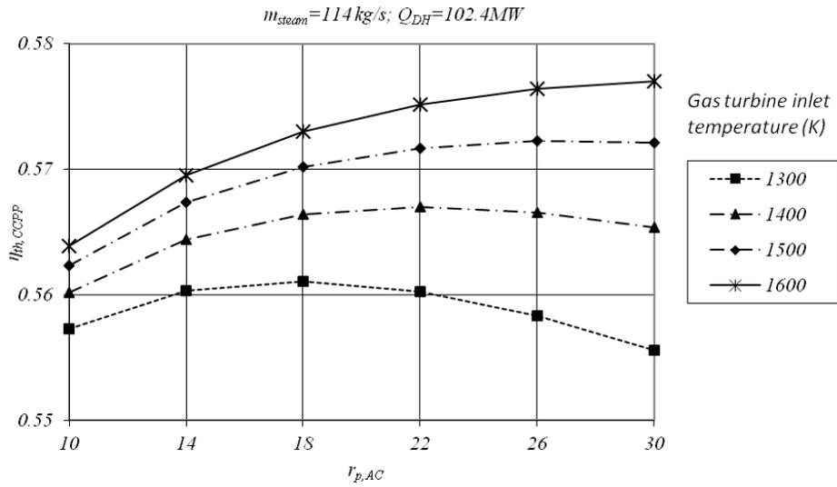
**Fig. 7** Thermal efficiency as a function of the compression ratio ( $r$ ) and the temperature of exhaust gases entering the gas turbine for 114 kg/s steam production and 102.4 MW heat output
