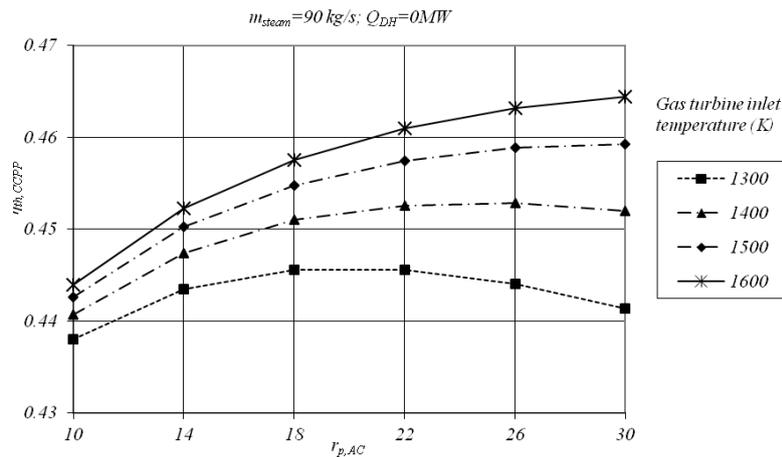
**Fig. 11** Thermal efficiency as a function of the compression ratio ( $r$ ) and the temperature of exhaust gases entering the gas turbine for 90 kg/s steam production and no heat output
