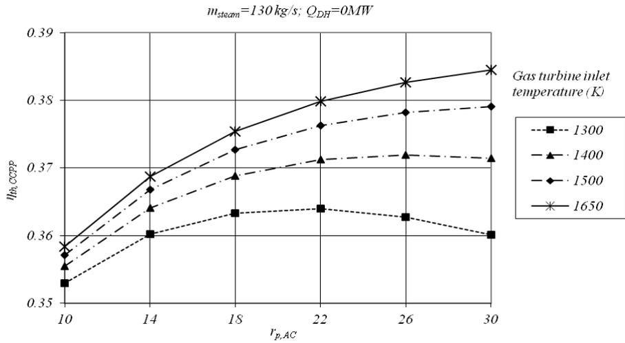
**Fig. 5** Thermal efficiency as a function of the compression ratio ( $r$ ) and the temperature of exhaust gases entering the gas turbine for 130 kg/s steam production and no heat output
