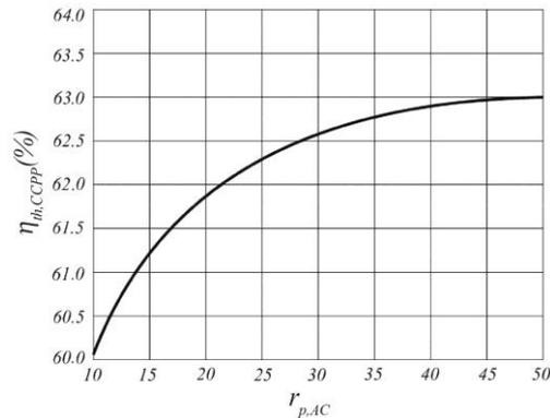
**Fig. 12** CHP thermal efficiency as a function of the compression ratio ( $r$ ) [27]
