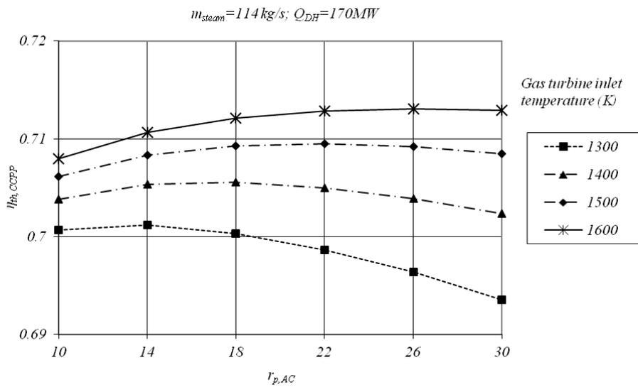
**Fig. 6** Thermal efficiency as a function of the compression ratio ( $r$ ) and the temperature of exhaust gases entering the gas turbine for 114 kg/s steam production and 170 MW heat output
