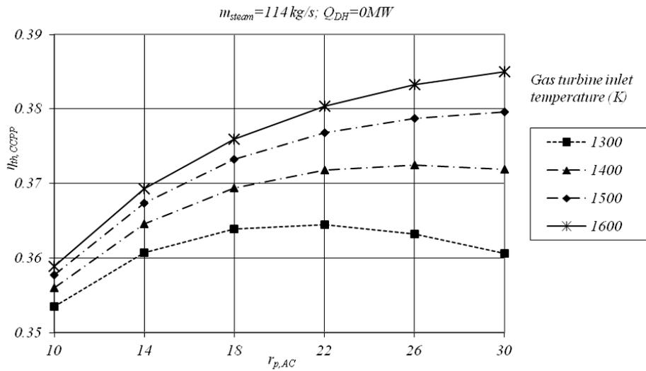
**Fig. 8** Thermal efficiency as a function of the compression ratio ( $r$ ) and the temperature of exhaust gases entering the gas turbine for 114 kg/s steam production and no heat output
