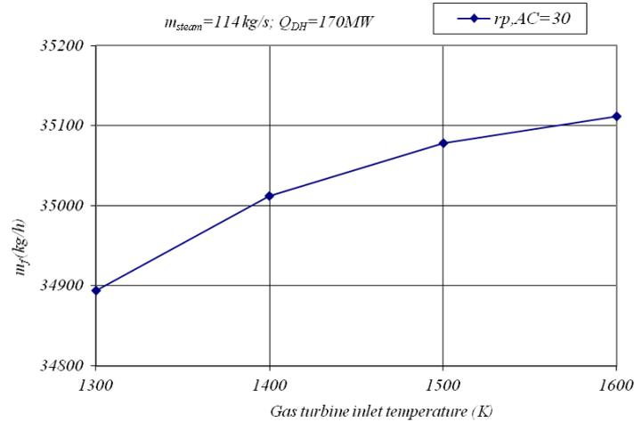
**Fig. 13** Fuel consumption as a function of the temperature of exhaust gases entering the gas turbine, for steam production of 114 kg/s and heat output of 170 MW
