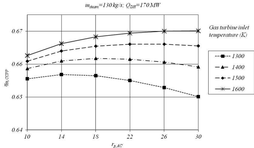
**Fig. 3** Thermal efficiency as a function of the compression ratio ( $r$ ) and the temperature of exhaust gases entering the gas turbine for 130 kg/s steam production and 170 MW heat output
