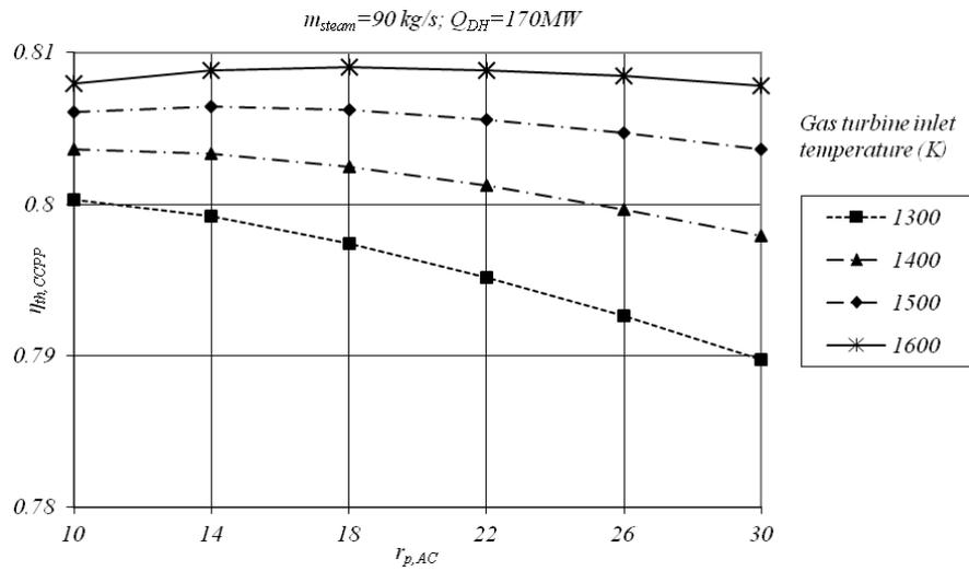
**Fig. 9** Thermal efficiency as a function of the compression ratio ( $r$ ) and the temperature of exhaust gases entering the gas turbine for 90 kg/s steam production and 170 MW heat output
