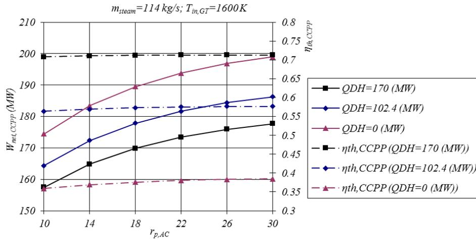
**Fig. 15** Electrical power output and thermal efficiency as a function of the compression ratio for steam production of 114 kg/s and entering temperature of 1600 K
