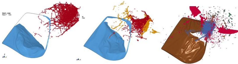
Fig. 5 Windshield deformations caused by a bird impact, left column – bird model, cylinder-shaped with spherical endings, middle column – bird model with a simplified shape, right column – real-life white stork bird model
