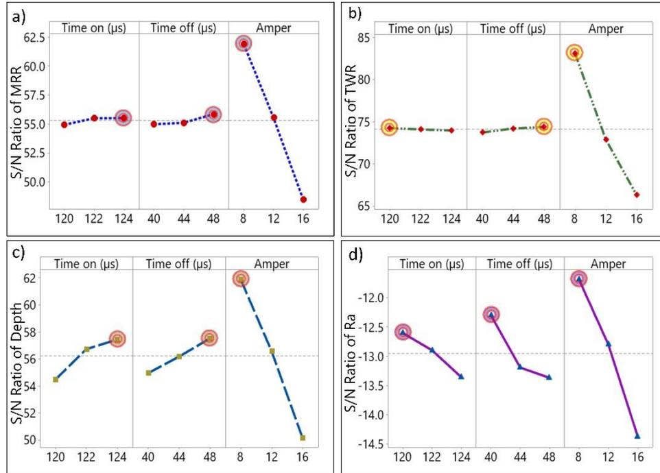
Fig. 5 Main effect plot for S/N ratio for a) MRR, b) TWR, c) Depth and d) Ra
