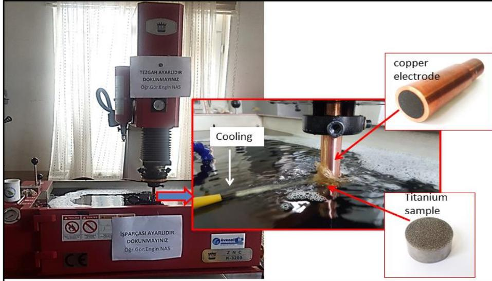
**Fig. 1** Electro-discharge machine used in the experimental work
