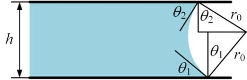
**Fig. 2** Geometry of a capillary bridge
