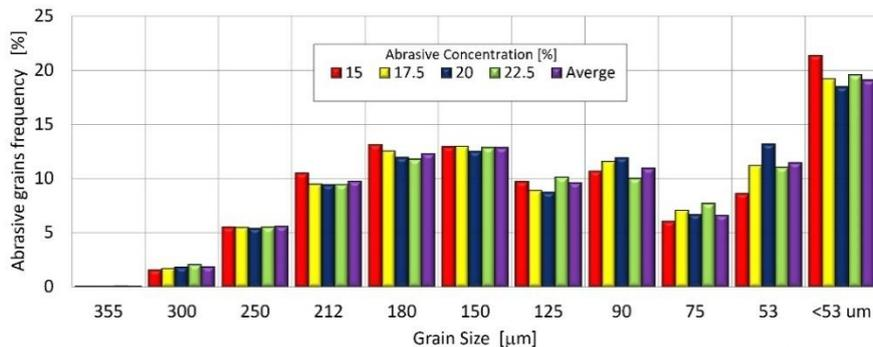
**Fig. 3** The disintegration of the effect of the GMA80 grain at water nozzle ID 0.33 mm, focusing tube ID 1.02 mm, and pressure 390 MPa
