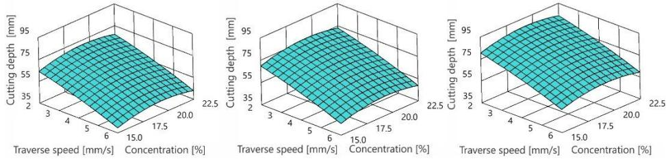
**Fig. 6** Effect of abrasive concentration and traverse speed on cutting depth with water nozzle diameter's: a) 0.25 mm, b) 0.29 mm, c) 0.33 mm
