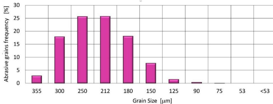
**Fig. 1** Typical GMA80 garnet grain size distribution
