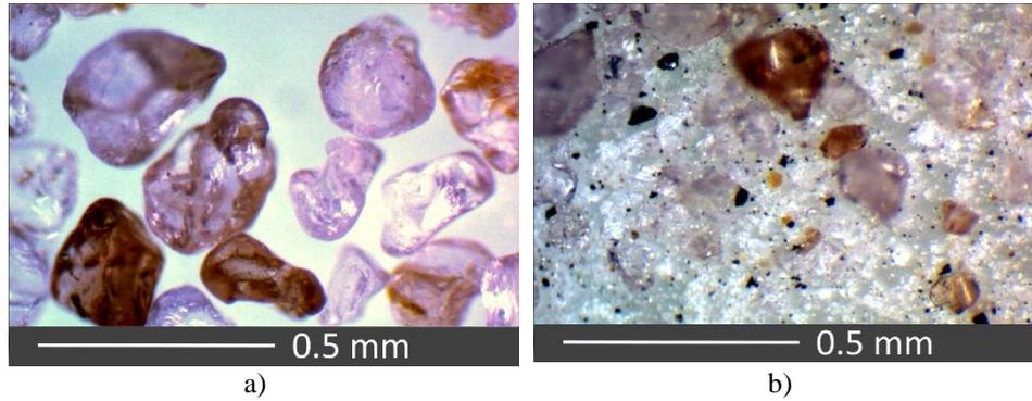
**Fig. 4** GMA80 abrasive grains a) fresh, b) after disintegration in the cutting head
