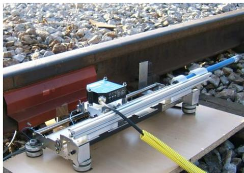
**Fig. 2** Laser device positioning relative to the rail
