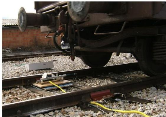
**Fig. 3** Trailing unit EMU 416-077– AOA measurement device without protective cover
