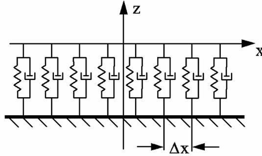
**Fig. 1** Equivalent one-dimensional visco-elastic foundation
