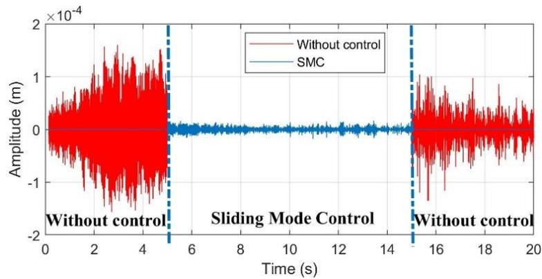
**Fig. 9** Data from controlled and uncontrolled situations
