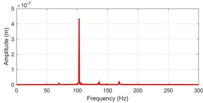
**Fig. 11** FFT results for displacement data without active control
