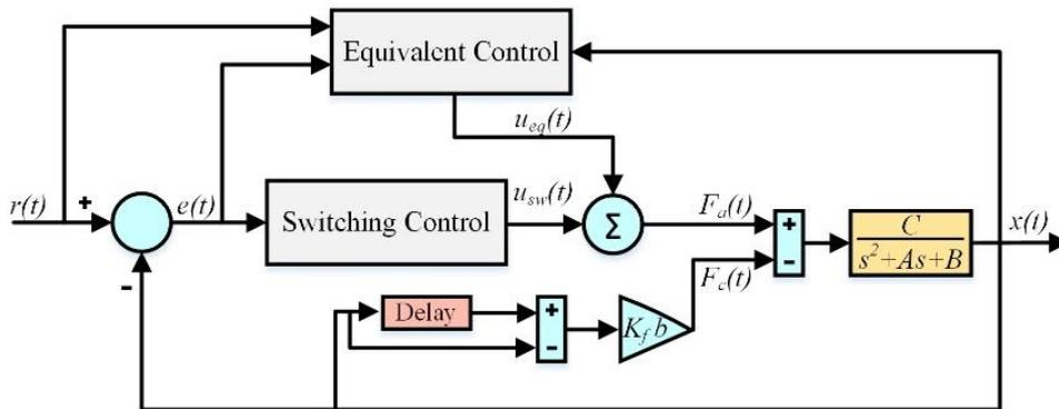
Fig. 4 SMC system block scheme
