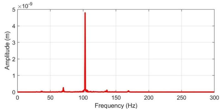
**Fig. 12** FFT results for displacement data after SMC
