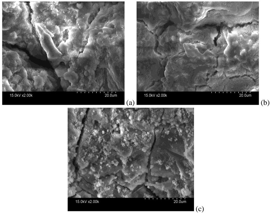
**Fig. 12** SEM micrographs of corroded surface (a) AZ31, (b) AZ31-2WC and (c) Polished sample
