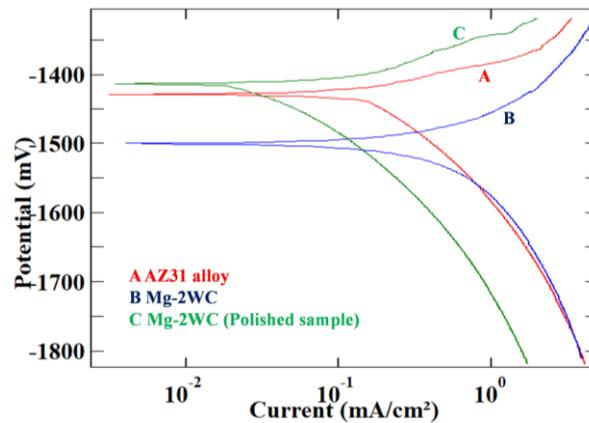
**Fig. 7** Potentiodynamic polarization plot for AZ31, AZ31-2WC and polished samples
