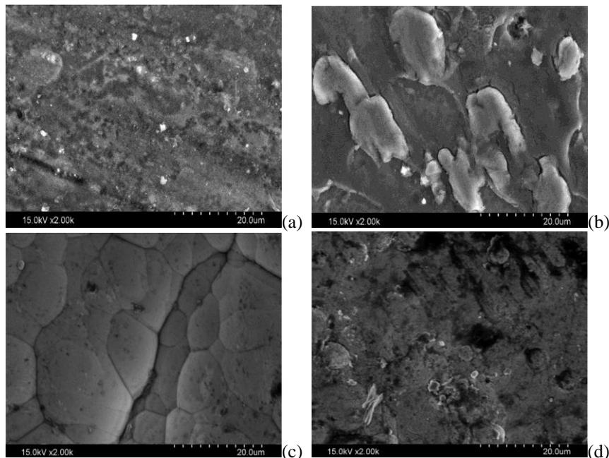
**Fig. 3** SEM micrograph (a) AZ31 alloy, (b) AZ31-2WC, (c) Ni-P coating and (d) Heat-treated Ni-P coating
