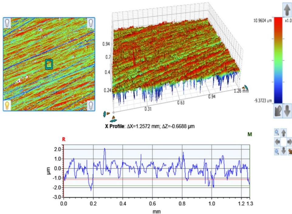
**Fig. 8** Surface roughness profile of polished AZ31-2WC sample
