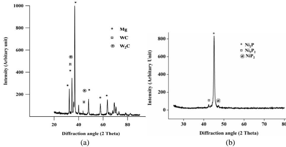
**Fig. 5** XRD plot (a) Mg-2WC nanocomposite and (b) Heat-treated coating sample
