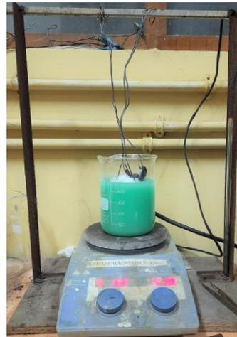
**Fig. 2** Pictorial view of coating deposition set up
