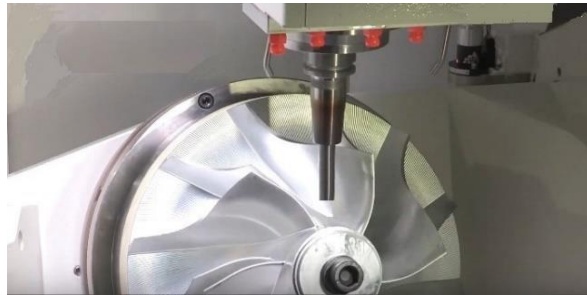
Fig. 9 The 5-axis milling operation of test impeller
