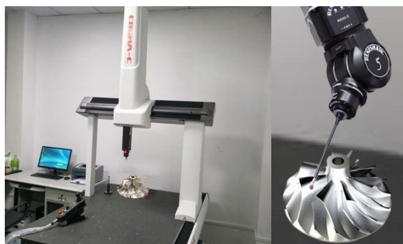
Fig. 11 The measuring process of the machined impeller blades using the CMM machine
