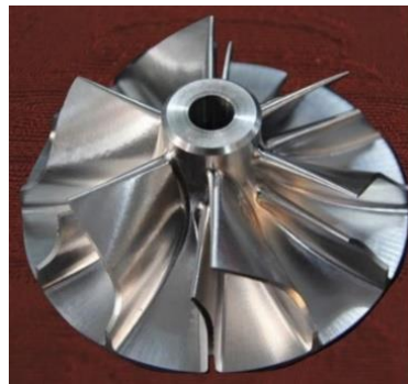
Fig. 10 The real machined AL impeller
