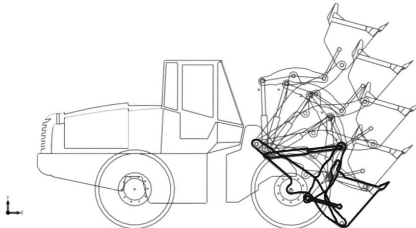
**Fig. 6** Simulation of the obtained optimal solution
