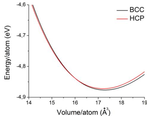
**Fig. 10** Energy per atom in HCP and BCC Ti crystallites with 13 at. % of vanadium as a function of atomic volume
