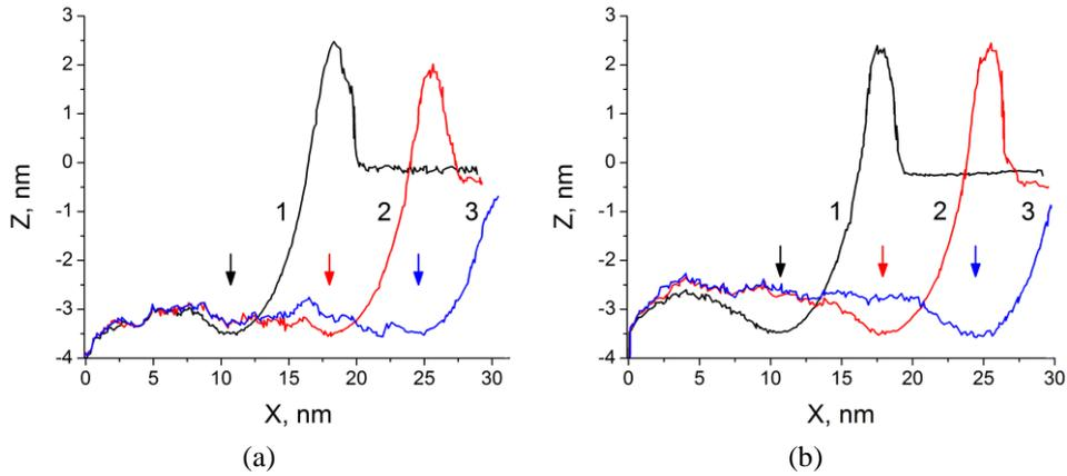
**Fig. 6** Longitudinal surface profiles of scratch grooves in (a) HCP and (b) BCC Ti crystallites after different scratching distances: 1 – 10.7 nm, 2 – 18.2 nm, 3 – 24.5 nm. Arrows indicate the position of the indenter center at the corresponding time points
