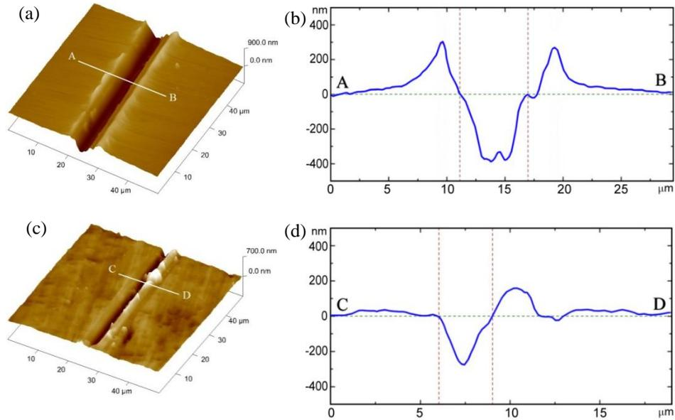
**Fig. 5** AFM-images (a, c) and corresponding cross-sectional surface profiles (b, d) of scratch grooves formed at the applied load 200 mN in (a, b) the as-built and (c, d) CEBS treated EBAM Ti-6Al-4V samples.
