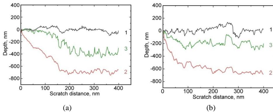
**Fig. 4** Longitudinal surface profiles of scratch grooves in (a) the as-built and (b) CEBS treated EBAM Ti-6Al-4V samples: 1 – initial surface profile, 2 – residual scratch profile, 3 – scratch profile at the applied load
