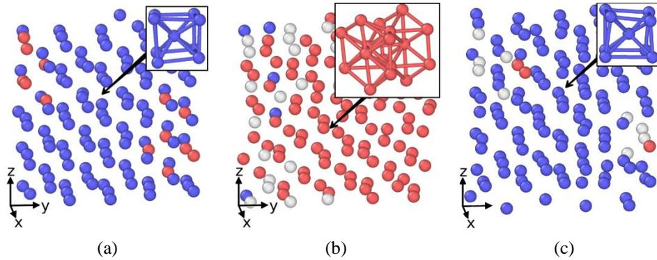
**Fig. 9** Evolution of the atomic structure of the fragment of BCC Ti crystallite during scratching: a – before loading; b – under compression induced by indenter; c – after unloading. BCC atoms are shown blue, HCP atoms are shown red, and atoms belonging to unidentified local configurations are shown grey
