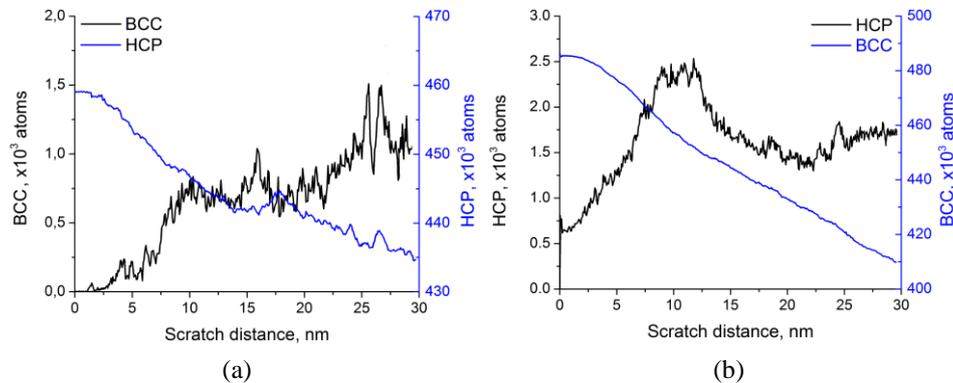
**Fig. 8** Number of atoms belonging to HCP and BCC crystal lattice in (a) HCP and (b) BCC Ti crystallites as a function of scratching distance. Atoms with non-identified type of ordering are not shown
