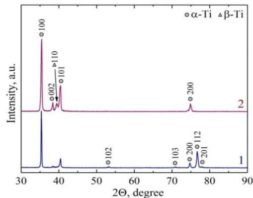
**Fig. 3** X-ray diffraction patterns of (1) the as-built and (2) CEBS treated Ti-6Al-4V samples
