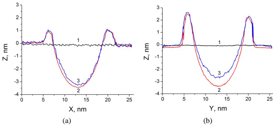
**Fig. 7** Cross-sectional surface profiles of scratch grooves in (a) HCP and (b) BCC Ti crystallites cut at  $X = 10.7$  nm at different points of loading: 1 – before loading, 2 – under loading (scratching distance is 10.7 nm), 3 – after unloading (scratching distance is 18.2 nm)
