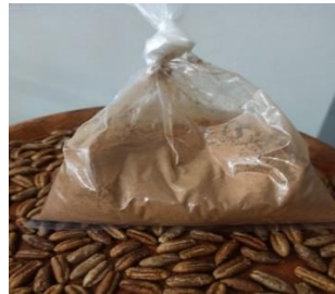
Fig. 2 Date seed after hammer milling in form of 200 µm spherical powder
