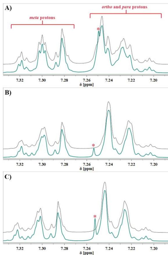
**Fig. 4** A comparison of the experimental (green) and simulated (gray) <sup>1</sup>H NMR spectra (the higher order phenyl group spin system) of phenethyl-angelate (A), -senecioate (B), and -tiglate (C). The residual solvent signal of CHCl<sub>3</sub> is designated with the symbol \*
