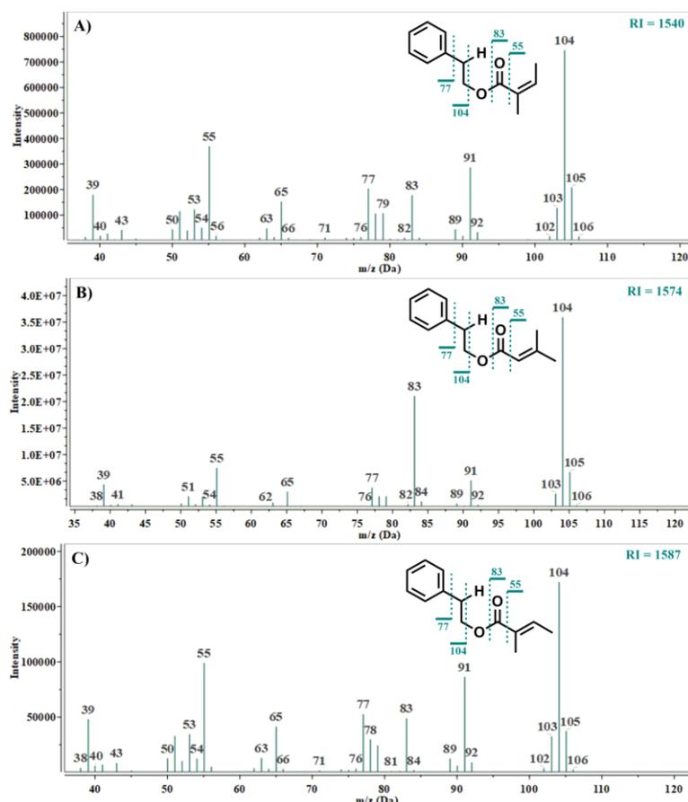
**Fig. 1** Comparison of MS spectra of phenethyl-angelate (**A**), -senecioate (**B**) and -tiglate (**C**) with the corresponding structures on which characteristic fragment ions are designated
