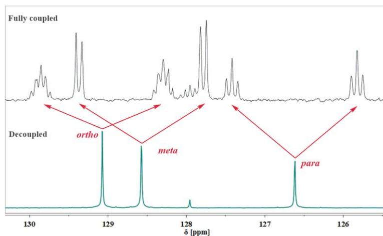
**Fig. 2** Fully  $^1\text{H}$  coupled and decoupled  $^{13}\text{C}$  NMR spectrum of phenethyl angelate (expansion of the region between 125.4 and 130.3 ppm) with designated signals of *ortho*, *meta*, and *para* carbons from the monosubstituted benzene ring
