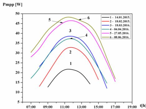
**Fig. 11** The results of the measurement of daily variations of maximum power  $P_{mpp}$  (W) of the horizontal solar module in the period from January to June.
