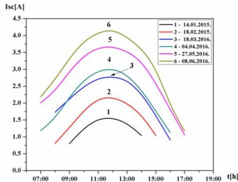
**Fig.7** The results of the measurement of daily variations of short circuit current  $I_{sc}$  (A) of the horizontal solar module in the period from January to June.
