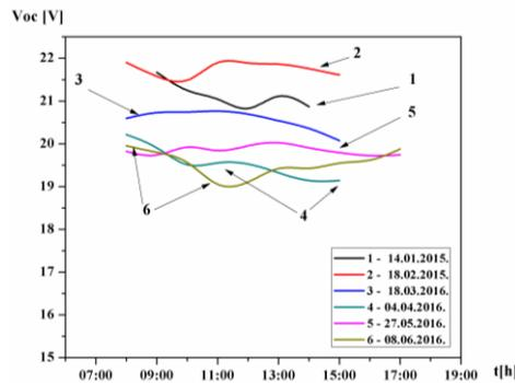
**Fig. 9** The results of the measurement of daily variations of open circuit voltage  $V_{oc}$  (V) of the horizontal solar module in the period from January to June.
