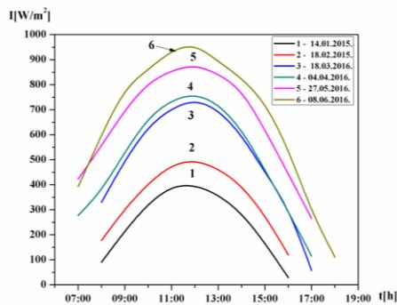
**Fig. 1** The results of the measurement of daily variations of the solar radiation intensity reaching the horizontal surface in the period from January to June.
