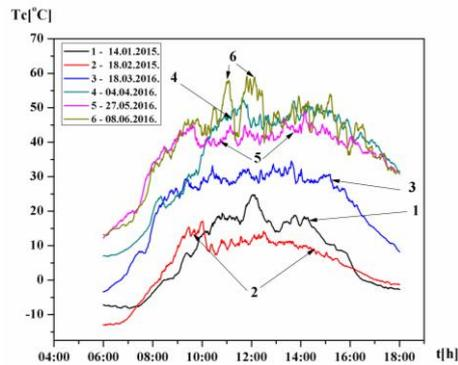
**Fig. 5** The results of the measurement of daily variations of the solar module temperature  $T_c$  in the period from January to June.
