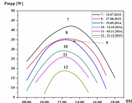
**Fig. 12** The results of the measurement of daily variations of maximum power  $P_{mpp}$  (W) of the horizontal solar module in the period from July to December.
