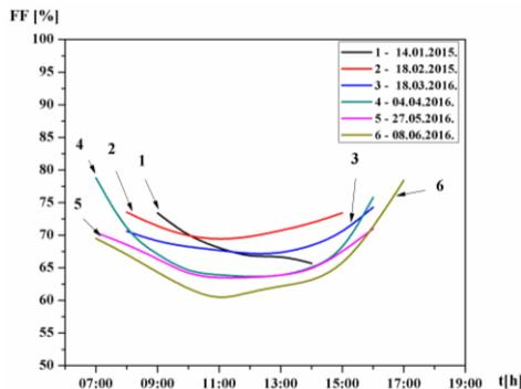
**Fig. 13** The results of the measurement of daily variations of fill factor  $FF$  (%) of the horizontal solar module in the period from January to June.
