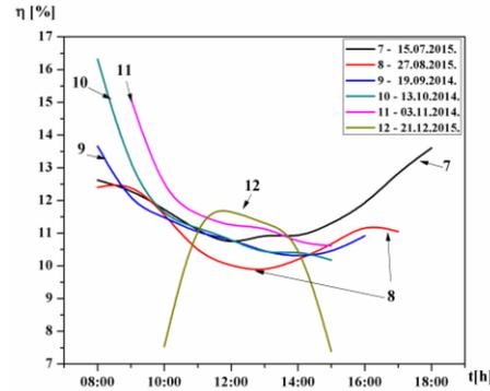
**Fig. 16** The results of the measurement of daily variations of the efficiency  $\eta$  (%) of the horizontal solar module in the period from July to December.
