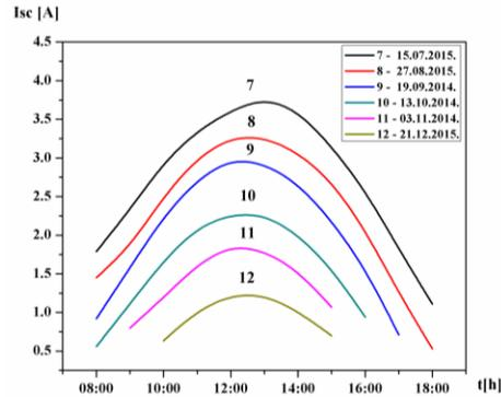
**Fig. 8** The results of the measurement of daily variations of short circuit current  $I_{sc}$  (A) of the horizontal solar module in the period from July to December.
