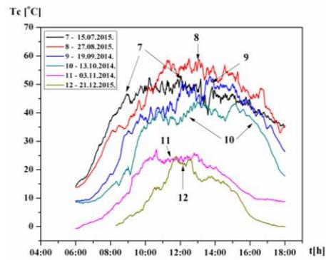
**Fig. 6** The results of the measurement of daily variations of the solar module temperature  $T_c$  in the period from July to December.
