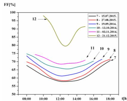
**Fig. 14** The results of the measurement of daily variations of fill factor  $FF$  (%) of the horizontal solar module in the period from July to December.
