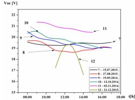
**Fig. 10** The results of the measurement of daily variations of open circuit voltage  $V_{oc}$  (V) of the horizontal solar module in the period from July to December.
