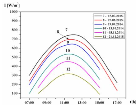
**Fig. 2** The results of the measurement of daily variations of the solar radiation intensity reaching the horizontal surface in the period from July to December.
