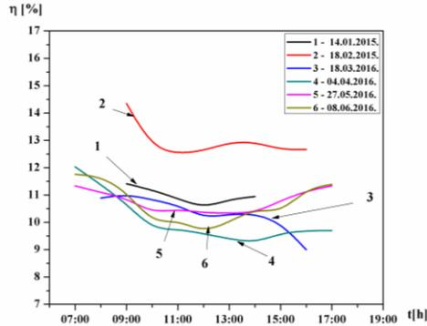
**Fig. 15** The results of the measurement of daily variations of the efficiency  $\eta$  (%) of the horizontal solar module in the period from January to June.
