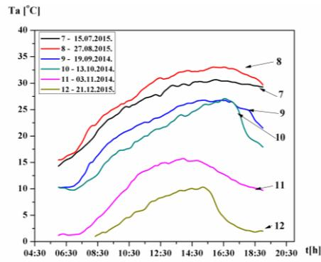
**Fig. 4** The results of the measurement of daily variations in the ambient temperature in the period from July to December.
