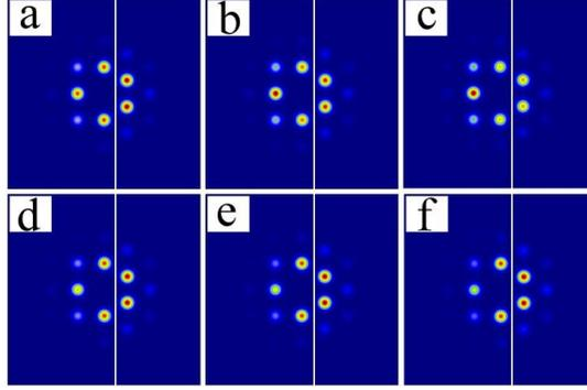
**Fig. 4** Surface vortex solitons at different lattice interfaces: (a)  $V_{0s}=2.51$ ,  $V_{0h}=2.5$ ; (b)  $V_{0s}=2.53$ ,  $V_{0h}=2.5$ ; (c)  $V_{0s}=2.55$ ,  $V_{0h}=2.5$ ; (d)  $V_{0s}=2.5$ ,  $V_{0h}=2.51$ ; (e)  $V_{0s}=2.5$ ,  $V_{0h}=2.53$ ; (f)  $V_{0s}=2.5$ ,  $V_{0h}=2.55$ .
