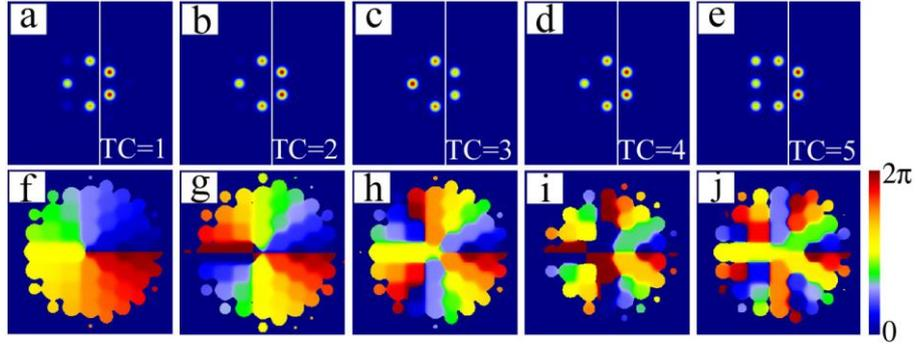
**Fig. 2** Five-lobe surface vortex solitons with different topological charges: intensity distributions (the first row) and corresponding phase distributions (the second row). Parameters:  $\mu=5.2$ , other parameters are as in Fig.1.
