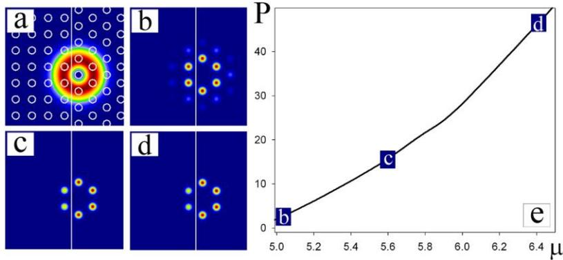
**Fig. 5** Surface vortex solitons with six lobes. Input vortex beam is shown at the lattice interface (a), with the layout of the lattice beams indicated by open circles. (e) Power diagram for the existence of six-lobe surface vortex solitons. The corresponding intensity distributions for different vortex solitons are presented in (b), (c) and (d); the lines depict the lattice interface. Parameters are as in Fig. 1.
