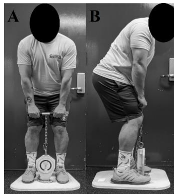
Fig. 1 Frontal (A) and sagittal (B) view of the set-up for the leg/back dynamometer test.
