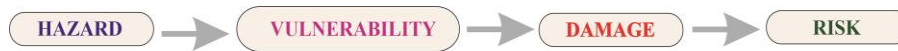
Fig. 1 Interconnection between hazard (hazardous event) and risk through vulnerability of an object and/or subject and the sustained damage
