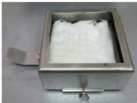
Fig. 4 Sample holder with ceramic fiber insulating material and retainer frame
