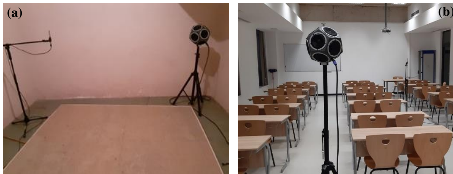
Fig. 2 Rooms where RIRs were measured: a) reverberation room, and b) classroom
