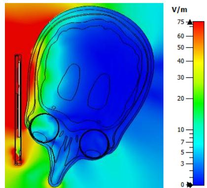
**Fig. 6** Electric field distribution within the user's head model – cross-section B
