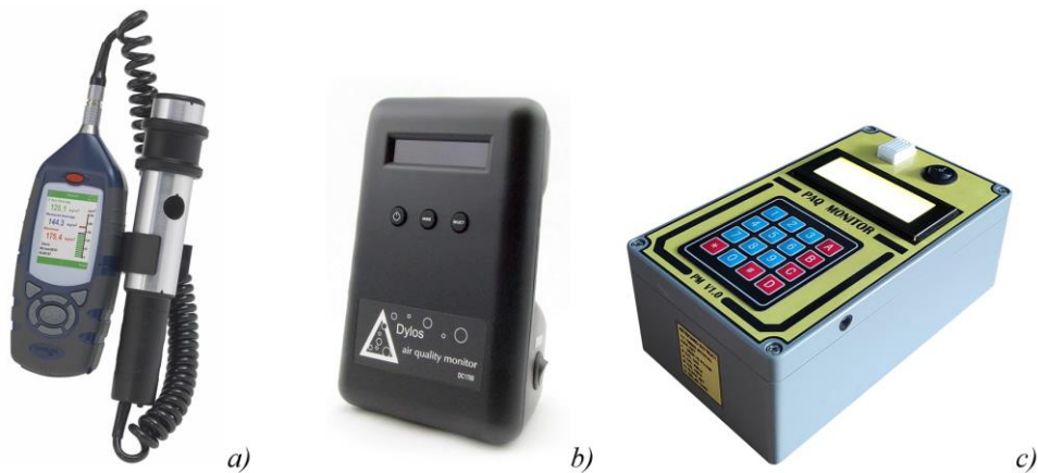
Fig. 1 (a) Casella Microdust Pro CEL-712, (b) Dylos DC1100 PRO (with PC interface), (c) PM V1.0 (with NOVA SDS011 sensor module) [10,11]
