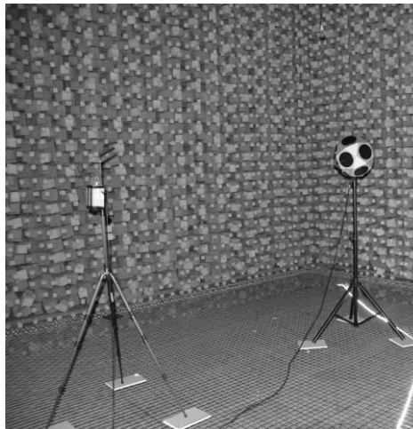
Fig. 3 The sound source and the PA measurement system at the anechoic room during the experiment
