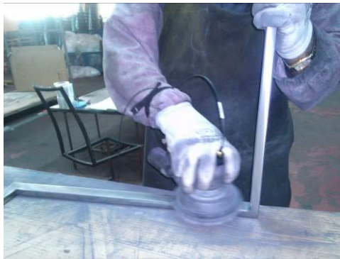
Fig. 8 Random orbital sander: the accelerometer attached by T-shape hand adaptor
