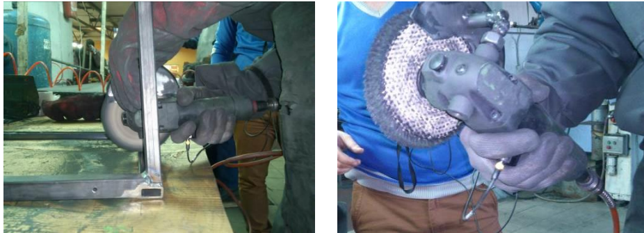
Fig. 9 a) Small angle grinder, b) The accelerometer attached by L-shape hand adaptor
