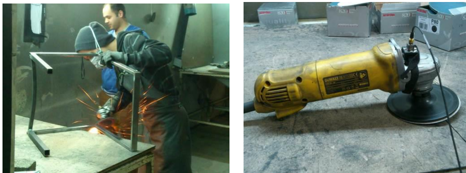
Fig. 10 a) Angle sander, b) The accelerometer attached by nylon strap
