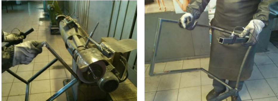
Fig. 12 a) Pedestal belt grinder, b) The accelerometer attached by nylon strap
