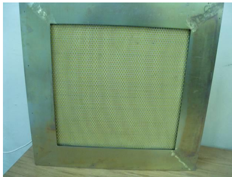
Fig. 3 Filter IPAF-2, view of the rear side reinforced by perforated foil
