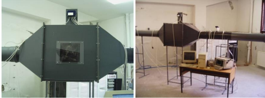
Fig. 1 Module of industrial air filter prototype and data acquisition system
