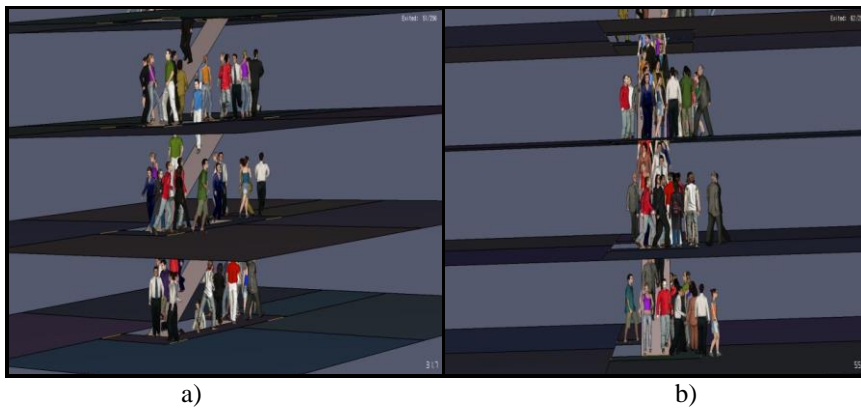
Fig. 8 Occupants are potentially stuck in case of different speed (a and b)
