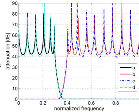
**Fig. 8** Attenuation of the high-pass filter including (a) and without  $\mu_i$  coefficients (c), and attenuation of the low-pass filter including (b) and without (d)  $\nu_i$  coefficients, respectively
