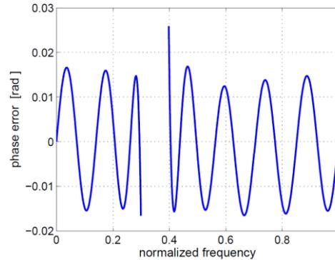
**Fig. 10** Phase error of the all-pass filter
