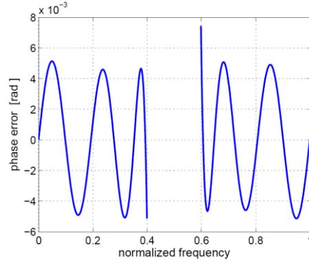
**Fig. 6** Phase error of the all-pass filter**Table 2** Poles of the all-pass filter
