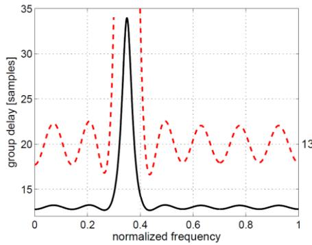
**Fig. 7** Group delay of the all-pass filter of order  $N=14$
