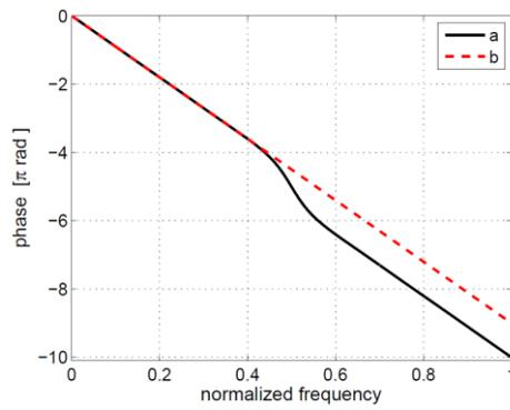
**Fig. 5** Phase of the all-pass filter (a) and phase of the delay line (b)
