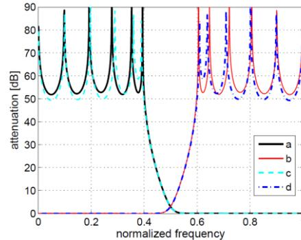
**Fig. 4** Attenuation of the high-pass filter including (a) and without  $\mu_i$  coefficients (c), and attenuation of the low-pass filter including (b) and without  $\nu_i$  coefficients, respectively
