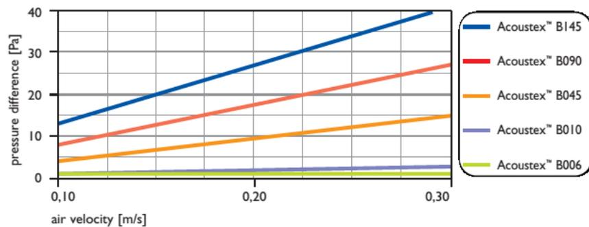
**Fig. 8** Dependence of the pressure drop for different types of materials
