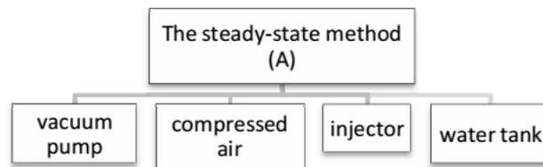
**Fig. 4** Ways of airflow supply in the steady-state method
