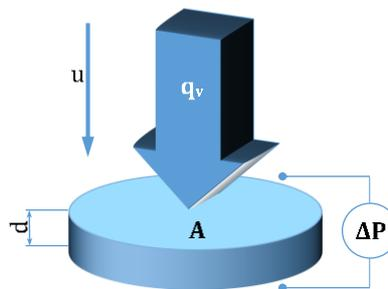
**Fig. 2** Schematic presentation of measuring airflow resistance
