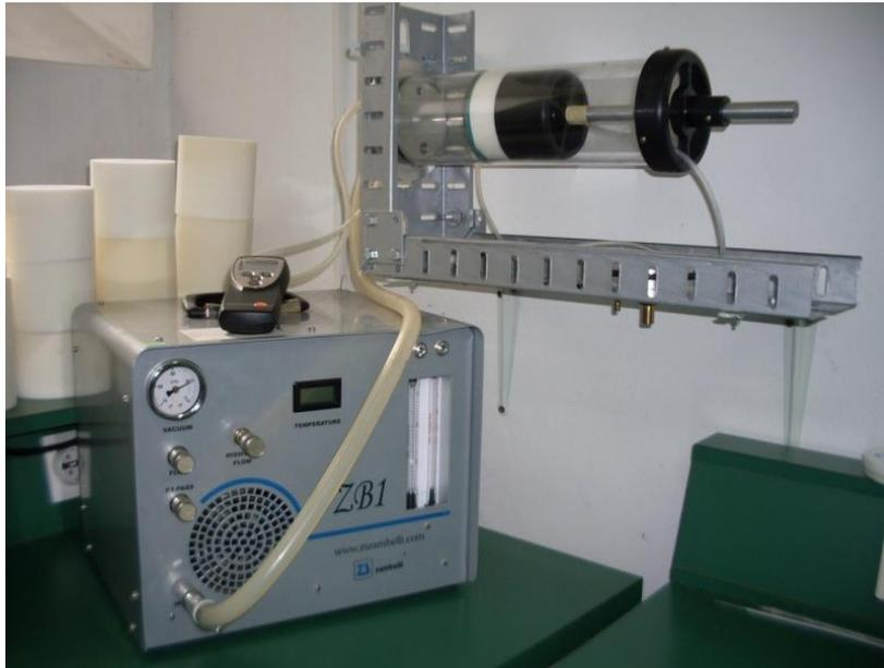
**Fig. 6** A view on the realized measurement system for determination of airflow resistance
