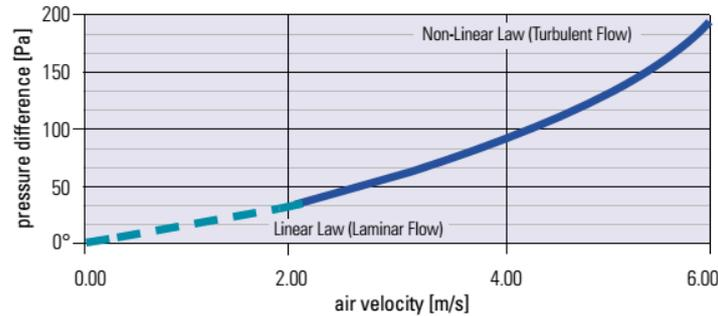
**Fig. 7** Airflow resistance – test conditions:
