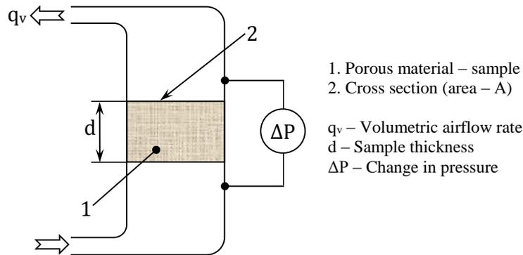
**Fig. 3** Steady-state method (method – A) – Basic principle
