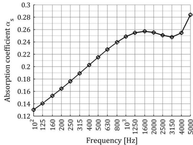
**Fig. 10** Sound absorption coefficient depending on the frequency
